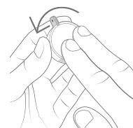
**EN** Open the key fob cover by turning it, and replace the battery.
