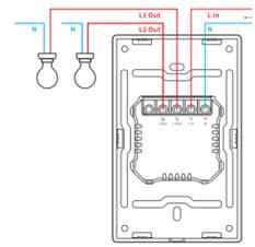
Make sure the neutral wire and live wire connection is correct.
