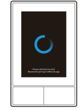
After powering on, the device will enter the Bluetooth Pairing Mode during the first use. The screen status is shown in the above image.
