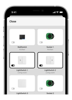
The lighting also can be controlled in the **Control** • menu. To do this, go to the **Control** • menu and swipe up. All control devices added to the hub will appear in the list. Click on the switch in the **LightSwitch** field, and the state of the device's contacts will change to the opposite. The lighting will be switched on or off.
