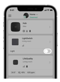
Click on the switch in the **LightSwitch** field in the **Devices** menu in the Ajax app, and the state of the switch contacts will change to the opposite. The lighting will be switched off or on. This way, system users can remotely control the lighting. For example, switch on the light in the room in advance before entering the room.
