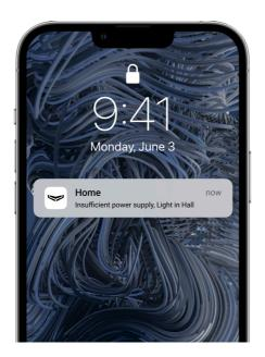
LightSwitch continuously checks its power supply parameters. If LightSwitch controls the power of a lighting device with insufficient power (up to 5 W), the system will notify the users of the Ajax system. In this case, it is necessary to replace the lighting device with a similar one with higher capacity or to connect a bundled capacitor in parallel with the lighting device.
