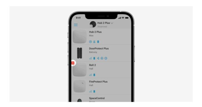
When the range extender detects a malfunction (for example, there is no external power supply), the Ajax app displays a badge with counter in the upper left corner of the device icon.
