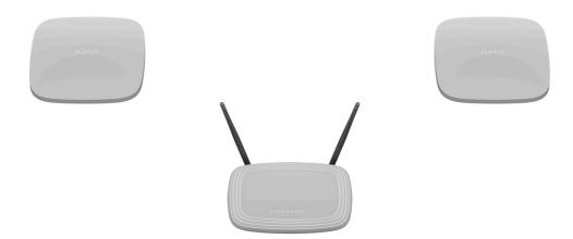
needed to determine the IP address for the range extender. The network to which ReX 2 Jeweller connects must allow broadcast queries and an open 4269 port for all types of traffic.
