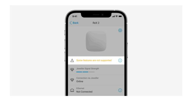
ReX 2 Jeweller can notify about malfunctions, if any. **Malfunctions** field is available in **Device States**. Clicking on (i) opens the list of all malfunctions. The field is displayed if a malfunction is detected.
